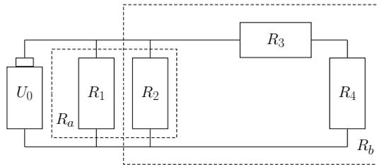
Calculate the voltage  $U_p$  provided by the battery if it has an internal resistance of  $r = \frac{R_1}{10} = \frac{R_2}{10} = \frac{R_3}{10} = \frac{R_4}{10} = 0.1 \Omega$  and a voltage of  $U_0 = 2 \text{ V}$ .
