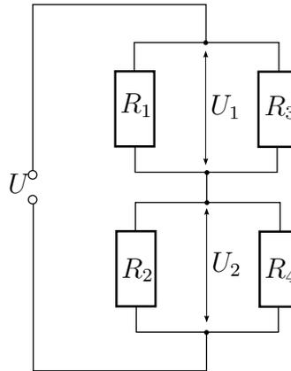
In the figure above it is  $R_1 = 10 \Omega$ ,  $R_2 = 20 \Omega$ ,  $R_3 = 50 \Omega$ ,  $R_4 = 100 \Omega$  and  $U = 24 \text{ V}$ .
